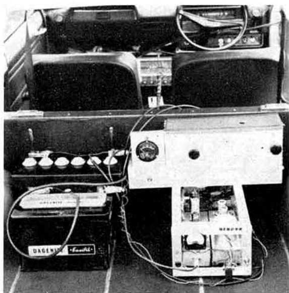
Internal arrangement. 70cm transmitter (top) and 2m transmitter each with own battery. Two connectors unite to effect "QSY to 70cm". The receiver below the parcel shelf can be seen between the seats
